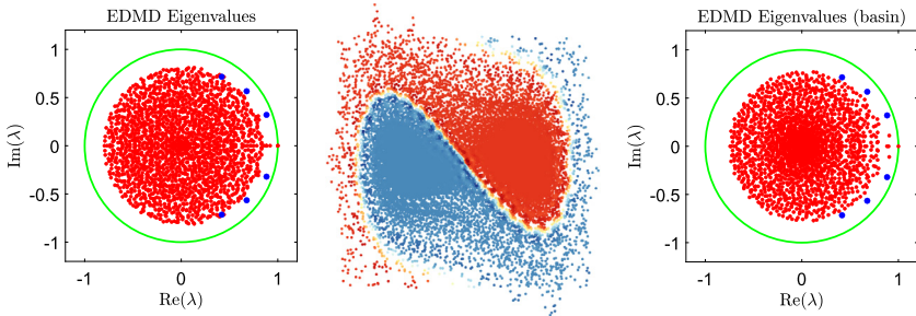
FIGURE 18 Left: EDMD eigenvalues computed over the entire state space. Middle: Eigenfunction that parametrizes the basins of attraction. Right: EDMD eigenvalues obtained after restricting the process to one basin of attraction. The powers of the dominant damped mode are shown in blue.
